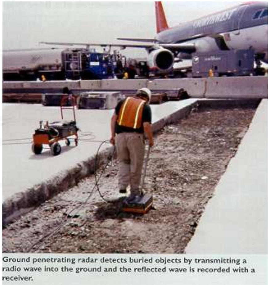
Ground penetrating radar detects buried objects by transmitting a radio wave into the ground and the reflected wave is recorded with a receiver.
